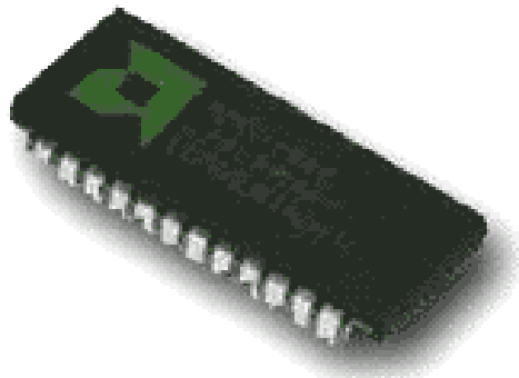
DIP (Dual Inline Package) Device (AMD Corporation)
